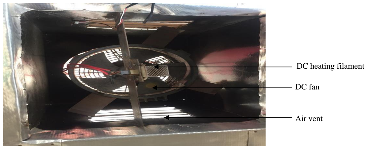
Figure 2: Hot-air supplement section of the dryer
